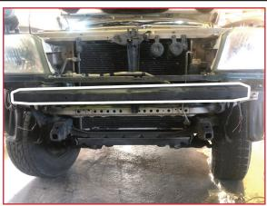
• Place the mounting winch bracket on the vehicle.
