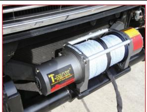
• Once the bar is on the vehicle, bolt the bulbar to the mounting bracket as seen in the image. do not over tighten.
