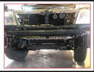
• Remove the steel beam running across the front of the chasis as shown in the image
