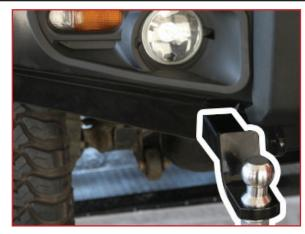
Tow hitch is used for off road use only, generally meant for pushing a trailer/caravan up driveways & the like. Not meant for on road use.
