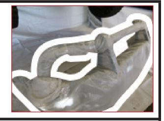
•Place the mounting winch bracket on the vehicle, Align the mounting holes on the side of chassis with bracket
