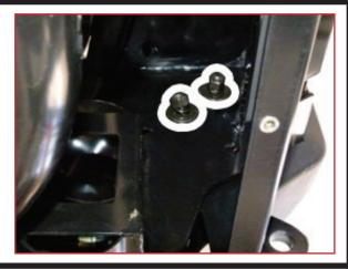
•Align the bar up with the vehicle, Insert tow hitches make sure they move in and out freely then tighten all the nuts on the mounting bracket and on the vehicle
