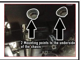
Note do not tighten the bolts until all the bolts have been mounted in there place
