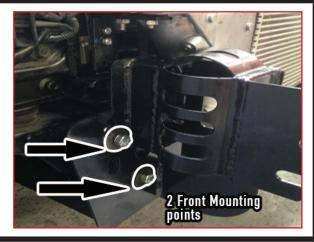
Once the bulbar has been unwrapped place the bar on the vehicle resting on the mounting bracket – NOTE if you are mounting a winch, this has to be done prior to mounting the bulbar on the bracket
