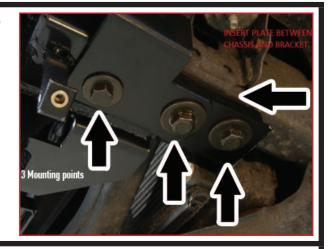
• The first point you have to insert the long bolt from the bottom to the top of the chassis.
