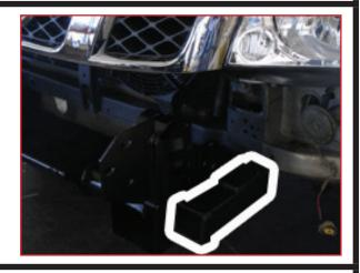
• Insert the plate reference picture above between the under body of the chassis and the mounting bracket.
