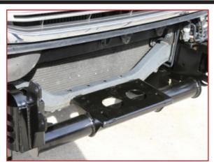
• When tow hitch is used, place the tow hitch on the same point as the bracket on the vehicle, if you are not using the tow hitch, skip this step (Tow hitch is an optional extra)
