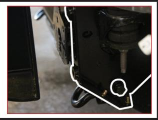
• Insert the plate with the capture bolt into the front of the chassis then fix into place as shown in the image, and secure it using a bolt.
