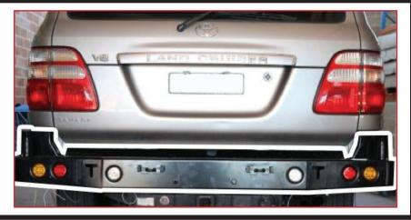
• All bolts should be mounted in on both side brackets once the bar is on the vehicle.
