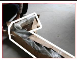
• Place the two side brackets on both side of the chassis as demonstrated in the photo, on some vehicles it may require the bracket to be spaced out slightly from the chassis this is due to different tow bars.
