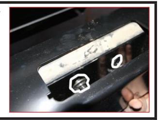
• Once all bolts are fastened, use the U shaped bracket and U bolt the bracket to the chassis.
