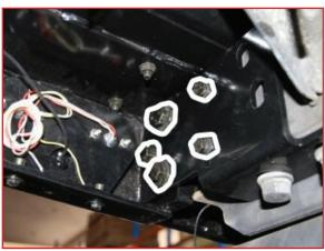
• Place the T Shaped nuts in to the chassis to allow the bolts from the side to fasten.
